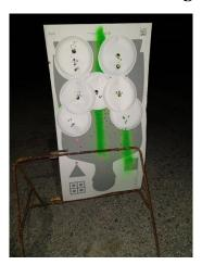
This can produce a dangerous situation as bullets can easily hit the crossbeam sending them in random directions, including back at the shooter. There definitely were signs of the crossbeam getting hit on this target stand.
