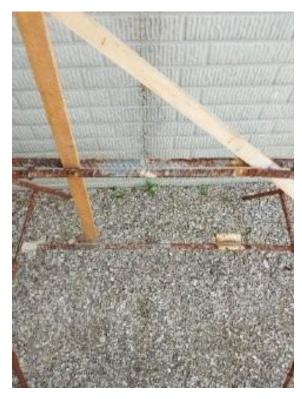
This metal stand and four others are missing the pry open handle used to install the laths. These are very hard to remove or install. Placing your target high above the stand will reduce damage to the steel stand.
